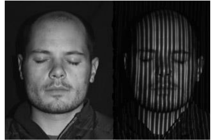
Visible structured light pattern (typically non-visible light is used).
